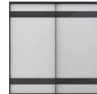
Panel: Top and bottom 120mm strip in the Smokey Mirror, rest of panels in Melteca Melamine Snowdrift Naturale.
